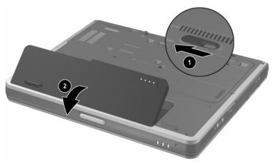
Removing the Battery Pack
